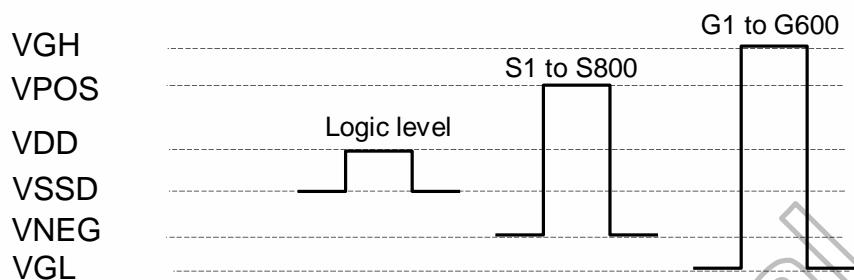
The logic levels of CLK, D[0:7], R/L, STH, LE, OE, CPV, U/D, MODE1, MODE2 and STV have to swing between VDD for "H" and VSSD for "L".
