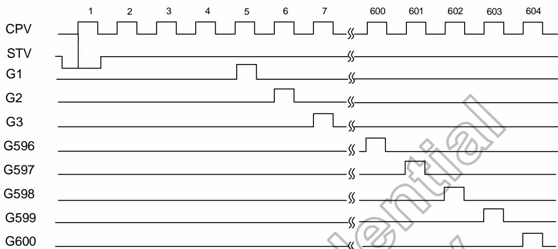
Example of input/output timing (U/D=L, MODE2=H, MODE1=H)
